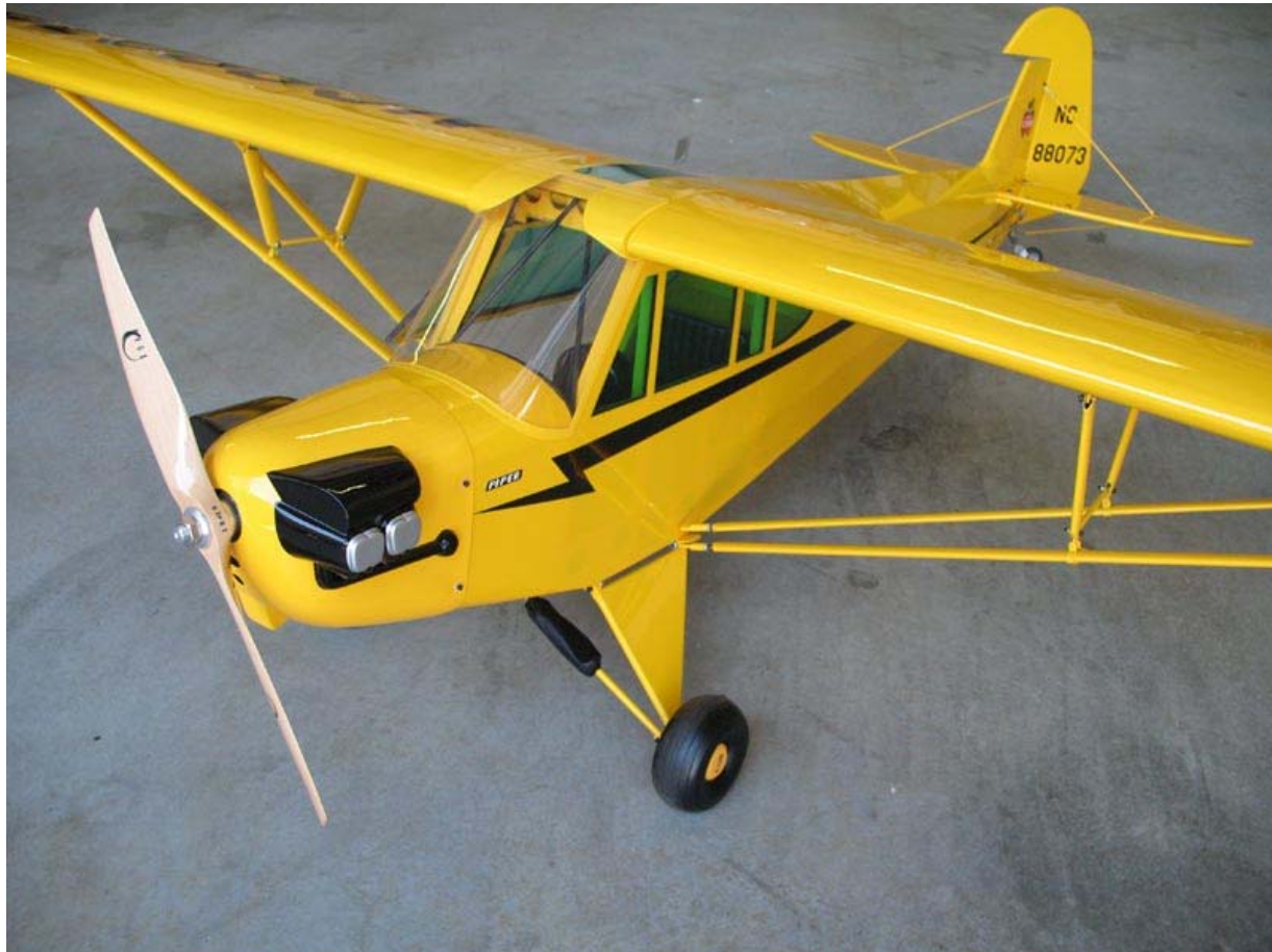
Figure 1. Horizon Hobbies Hangar 9 “Quarter-Scale Piper Cub” UAS
